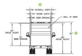
The box dimensions and configurations on this page represent a standard dry freight box. The liftgate as pictured is an option and not part of the standard configuration.
